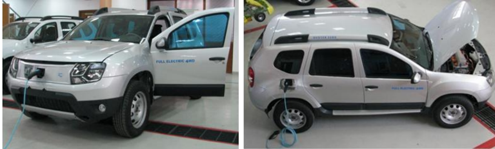
Figure 11. The front socket (left) and rear socket (right) for DUSTER ZERO 4WD [2]
