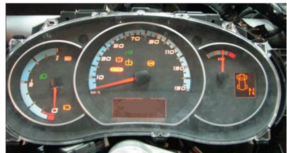
Figure 9. The DUSTER Z.E.RO 4WD cockpit and dashboard with the charge level of the traction battery (left); speed indicator (centre); econometer (right) [2, 3]
