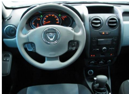
Figure 9. The DUSTER Z.E.RO 4WD cockpit and dashboard with the charge level of the traction battery (left); speed indicator (centre); econometer (right) [2, 3]
