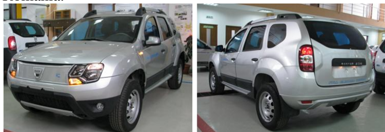
Figure 1. DUSTER Z.E.RO (ZERO- Z ero E mission R omanian concept) a full electric 4WD vehicle developed within the Automotive Engineering Research Centre, University of Pitesti [1, 2, 3]
