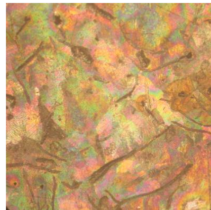
Figure 5. Cast Iron lamellar graphite microstructure (scale x200)
