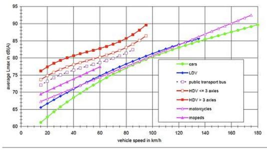
Figure 2. Road noise level depending on the speed and type of vehicle [16].
