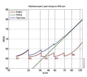
Figure 1. Road n20oise level depending on vehicle speed, at constant speed [15].
