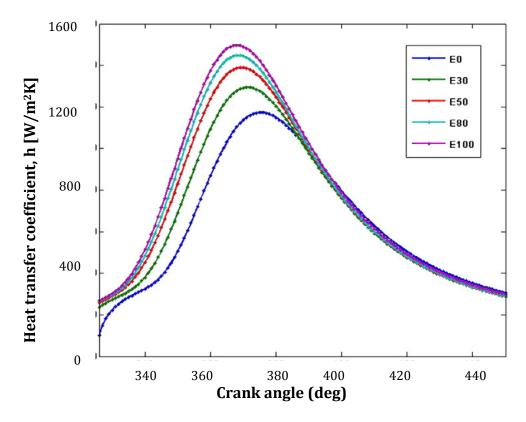
Figure 6. Coefficient of heat transfer vs. crank angle for different ethanol–gasoline blends [6]
