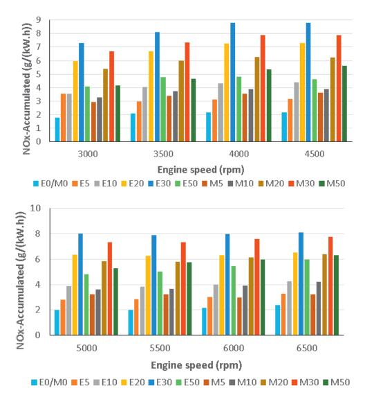
Figure 7. Influence of ethanol and methanol gasoline blended fuels on NOx emissions. [9]
