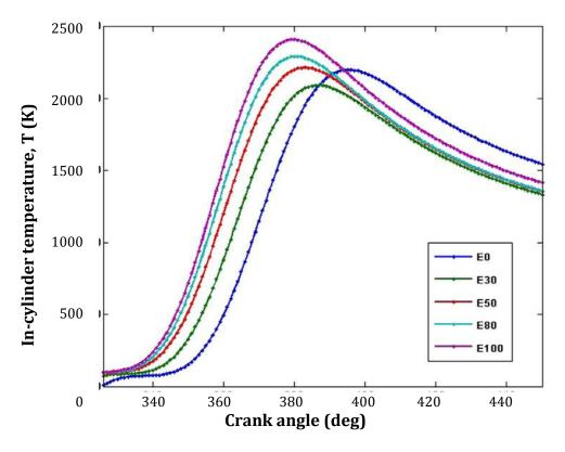
Figure 4. In-cylinder temperature against the crank angle for different ethanol-gasoline blends [6]
