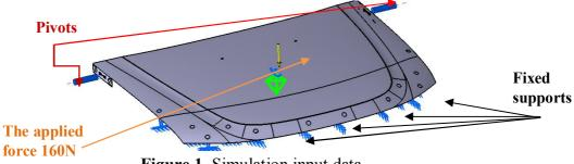
Figure 1. Simulation input data
