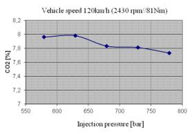
**Figure 4.** CO<sub>2</sub> emissions in percentages depending on the injection pressure for the vehicle speed of120km/h
