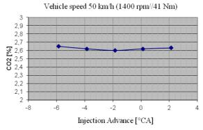
Figure 3.  $CO_2$  emissions in percentages depending on the modification of the injection advance for the vehicle speed of 50 km/h
