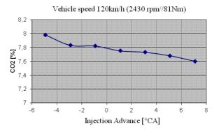
Figure 5.  $CO_2$  emissions in percentages depending on the modification of the injection advance for the vehicle speed of 120km/h
