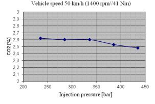
Figure 2.  $CO_2$  emissions in percentages depending on the injection pressure
