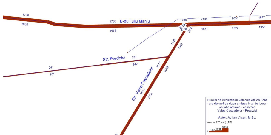
Figure 1. Traffic flows at the PM (post-meridian) peak hour after the model up-dating and up-grading for the current conditions.
