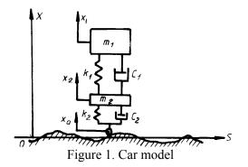
Study using the model of the car with two degrees of freedom in Figure 1 and analytical method for assessing the quality of vehicle suspension, frequency response and root mean square response (transmissibility) system, to obtain indicators for assessing the sensitivity factors for excitation system and mode of transmission of the phenomenon analyzed.
