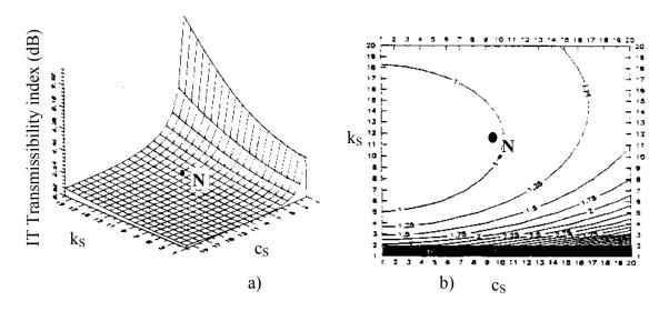
Figure 7. Three-dimensional coordinates obtained by changing simultaneously the surface coefficient of spring stiffness and damping coefficient  $\mathbf{k}_s$ ;  $\mathbf{c}_s$ .
