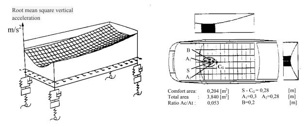
Figure 8. Values transmissibility function of vertical acceleration
