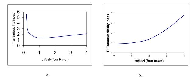
Figure 6. Transmissibility index vs. damping and stiffness
