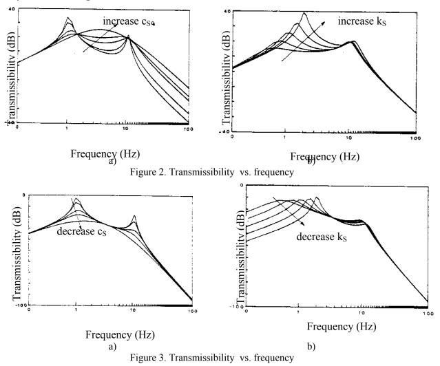
The influence of suspension stiffness changes on transmissibility diagama shown in figure 3, where it notes that, to increase damping decreases the transmissibility (Fig.a) and the (fig.b) observed that with increasing stiffness suspesiei strong amplification occurs and also a shift of its maximum under the first mode of vibration in the 4-10 Hz and 2-3 Hz in the high frequency area, there is mitigation.
