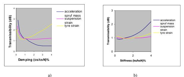
Figure 5. Transmissibility vs. damping and stiffness
