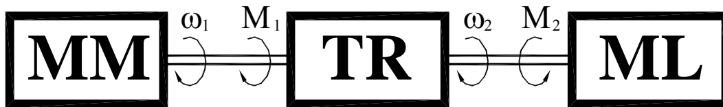
Figure 1. The scheme of the drive system
