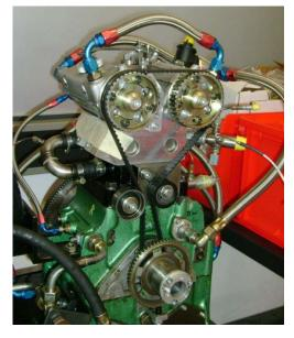
This engine has been equipped with a specific electro-hydraulic system on the exhaust valve to realize a second opening of the valve (the so called "re-breathing") during the intake stroke so as to provide high rate of residual gas in the combustion chamber for auto-ignition operation (Fig. 4).
