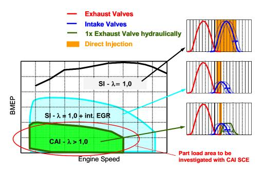
Figure 5. Operation strategy for CAI single cylinder engine
