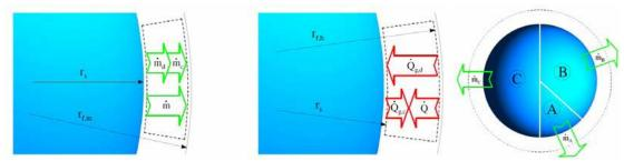
Figure 1. Mass and Heat Fluxes for Multi-component Droplet
