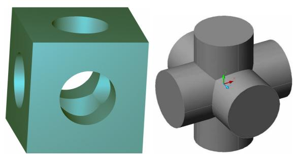
Fig. 1. Spatial representation of the exterior and interior of the explosion bomb.
