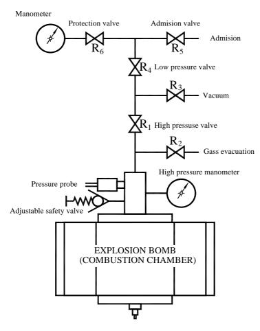
Fig. 2. Hydraulic scheme of the explosion bomb.
