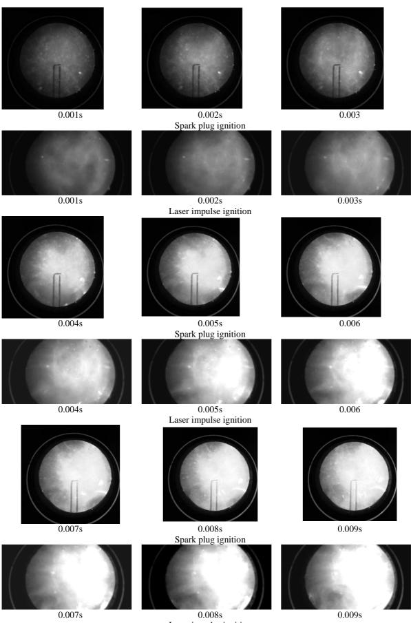
Laser impulse ignition Fig. 7. Frames from the recordings done with the rapid camera.
