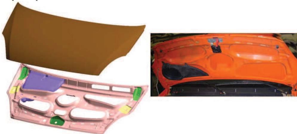
Fig. 10. An exploded view of the reference bonnet solution of a light commercial vehicle (on the left) and a photograph with a front view of the opened bonnet (on the right)
