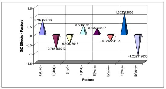
Fig.1 The adjusted technological parameters effect  $(U_a, I_s, v_s \notin v_e)$  on the signal/ noise ratio For the welding belt shape coefficient  $\psi$
