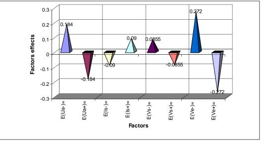
Fig.2 the adjusted technological parameters effects  $(U_a, I_s, v_s \notin v_e)$  on the measured Sizes for the welding belt shape coefficient  $\psi$
