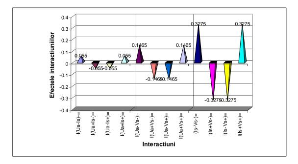
Fig.4 the adjusted technological parameters effects  $(U_a, I_s, v_s)$  on the measured sizes R for the welding belt shape coefficient  $\psi$
