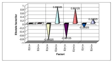
Fig.3. Effects of the technological adjusted parameters (t, s, n, r) on the Signal/Noise ratio for the  $R_{7ISO}$  roughness of the processed surfaces.
