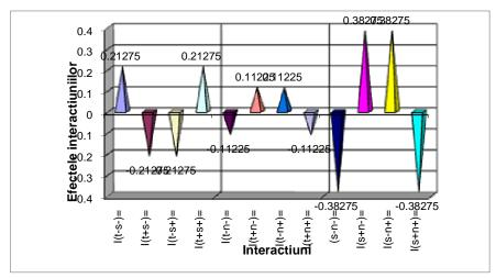
Fig.4. Effects of the interaction of the technological adjusted parameters (t, s, n, r) on the Signal/Noise ratio for the  $R_{zISO}$  roughness of the processed surfaces.
