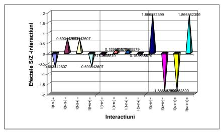
Fig.2. Effects of the interaction of the technological adjusted parameters (t, s, n, r) on the Signal/Noise ratio for the  $R_{zISO}$  roughness of the processed surfaces.
