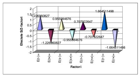
Fig.1 Effects of the technological adjusted parameters (t, s, n, r) on the Signal/Noise ratio for the  $R_{zISO}$  roughness of the processed surfaces.
