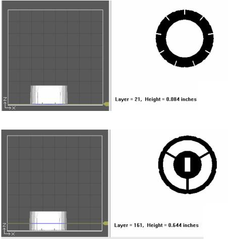
Fig. 4. Example of cross sections on the virtual model
