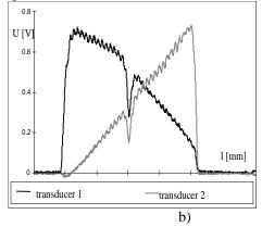
Fig. 2. Variation of the signal given by the resistive transducers during processing a)  $ZrO_2$ ; b)  $Al_2O_3$  As it can be noticed from the analysis of the Fig. 2.a), in the case of processing  $ZrO_2$  the two transducers work almost symmetrical, as the ceramic plate used for determinations, with the sizes  $80 \times$
