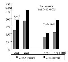
Fig. 4. Dependency of the conventional constituent values of the cutting force to the grinding conditions  $(v_d, v_p \text{ and } t)$ , for  $ZrO_2$  processing
