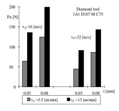
Fig. 5. Dependency of the conventional constituent values of the cutting force to the grinding conditions parameters  $(v_d, v_p \text{ and } t)$ , for  $Al_2O_3$  processing
