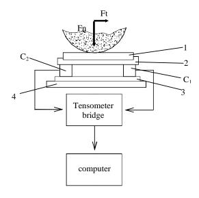
Fig. 1. Block-diagram of the mounting used for measuring the grinding force constituents
