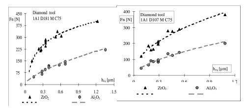
Fig. 3 The variation of the conventional constituent of the cutting force function of the  $h_{\rm eq}$
