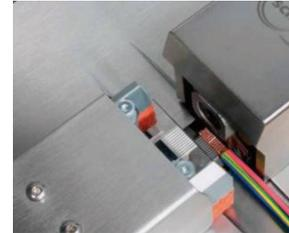
Fig. 3 Welding operation with ultrasounds
