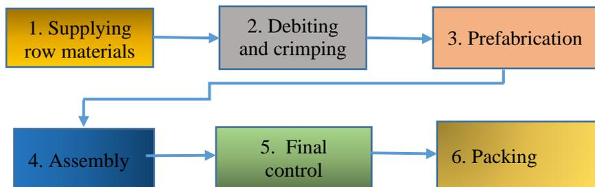
**Fig.1** The manufacturing process of a car wiring – main stages
